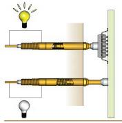
A wide area of applications is possible with the switching probes. When pressing the plunger the circuit is closed in the probe. Thus, the presence of components, open/closed checks and many more can be realised for instance.
