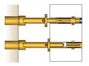
Step probes are inserted in the connector housings to test the correct position of the contact terminal (contact sheets). A contact will only be produced by the pin of the step probe when it is correctly positioned.
