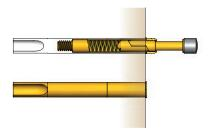
To transmit high currents, such as in function tests, high current probes are used. Due to their design, high current test probes have a very low internal resistance and warm only very slightly when loaded.
