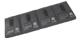
For production operation, Superpro 501S N\*Cluster operates in stand-alone (without a PC attached) mode. Each unit supports manufactures including EPROM, EEPROM and Flash memory, PIC, AVR and other popular microcontrollers and PLDs. By operating multiple programmers simultaneously you can use them in high volume production environment
