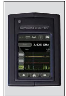
The frequency adjust screen displays Transmit, 2nd, or 3rd frequency ranges.
